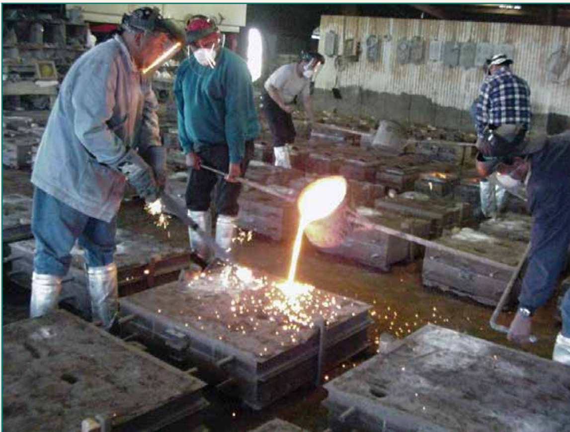
Some of the HCID2 crew pouring molten metal at the foundry.
