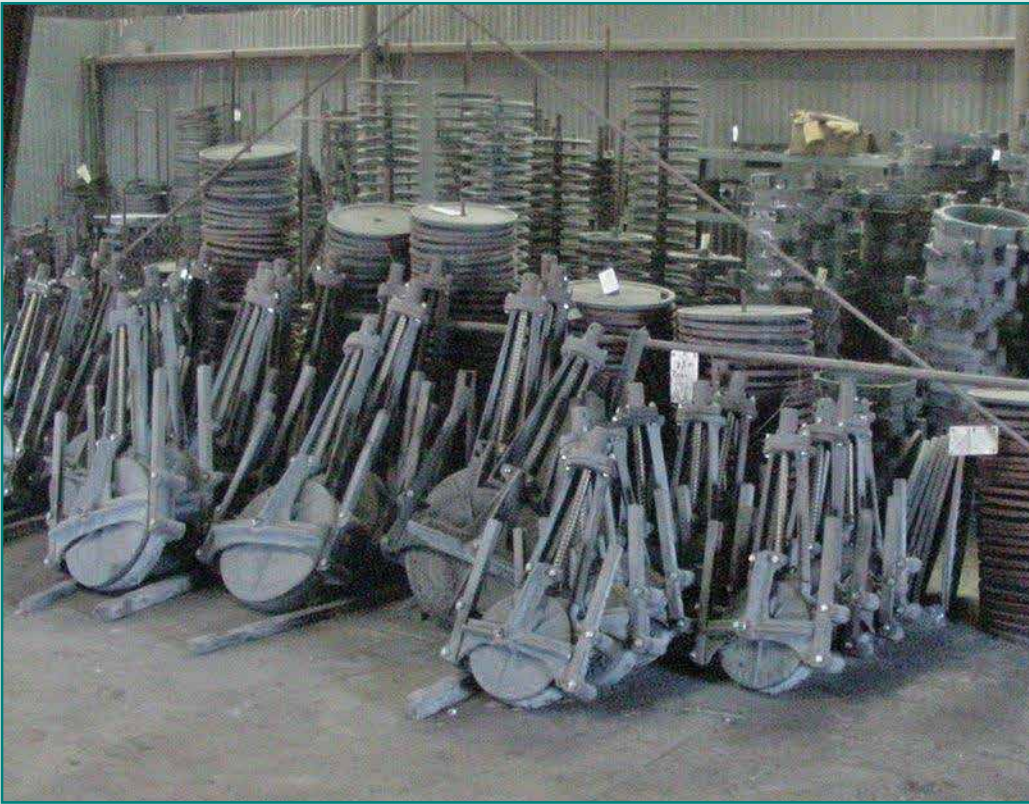
Well gates forged at the HCID2 foundry.
